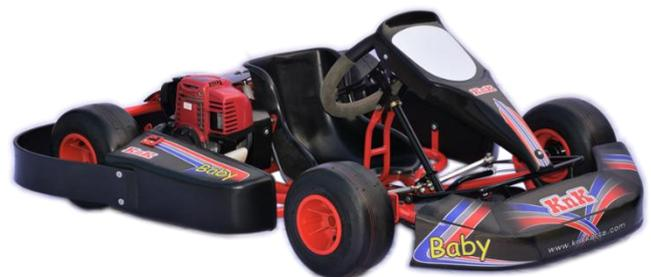
It is driven by a reliable and high revving Honda GX35 OHC engine.
