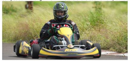
Kart that won a Canadian 4 stroke National championship in 2010. Exclusively built for 4 stroke racing, powered by a race prepared Honda GX200 TAG Engine producing around 11 bhp, this highly tunable chassis makes it easy to race and setup for different tracks and conditions.
