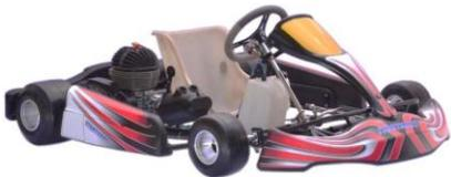
The STARTKART models are built on proven KnK Juvenile, Integra and JL chassis', they cover all age segments and offer engine packages starting with 4-stroke from 6.5 bhp through to 28 bhp 2 stroke engines. The 4-stroke model chassis' permit upgrading to 2-stroke at minimal costs.
