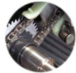
Plastic chain tension slippers – smooth efficacy
