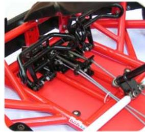
Adjustable pedal and steering positions for drivers of different Heights.
